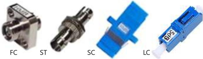
The Fixed Adapter Type Attenuator, also known as the Fixed Bulkhead Type or Fixed Female-Female Optical Attenuator, is a passive device that reduces the power of optical signals in fiber optic systems. It utilizes the air gap between two connectors to achieve the optical attenuation, making it a simple, low-cost, and compact solution for applications where return loss is not a concern.
