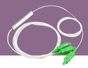
The Fiber Optic Ratio Splitter, also known as a fiber optic coupler, is a device designed for power distribution and tapping in optical fiber amplifier, online monitoring system, PON (passive optical network), OCT medical imaging, and CATV solutions. It is capable of distributing or combining optical power among different optical fibers by a certain coupling ratio.
