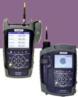
In addition to providing a full day of battery-operated field use, the SmartClass Fiber OLP-85 and -85P are perfect for fixed installations in central offices, production environments, and for laboratory workbenches because they can operate via mains or be remotely controlled via USB 2.0 and Ethernet.
