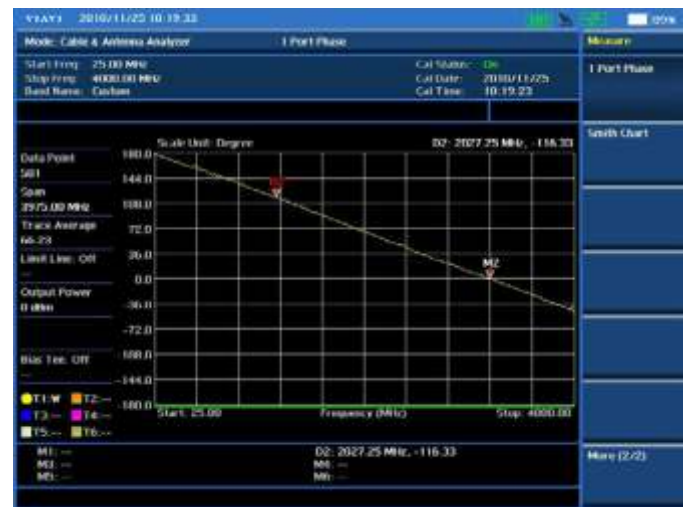
Cable and antenna test — 1-Port Phase
