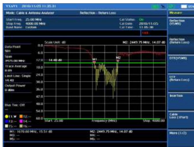
Cable and antenna test — Reflection
