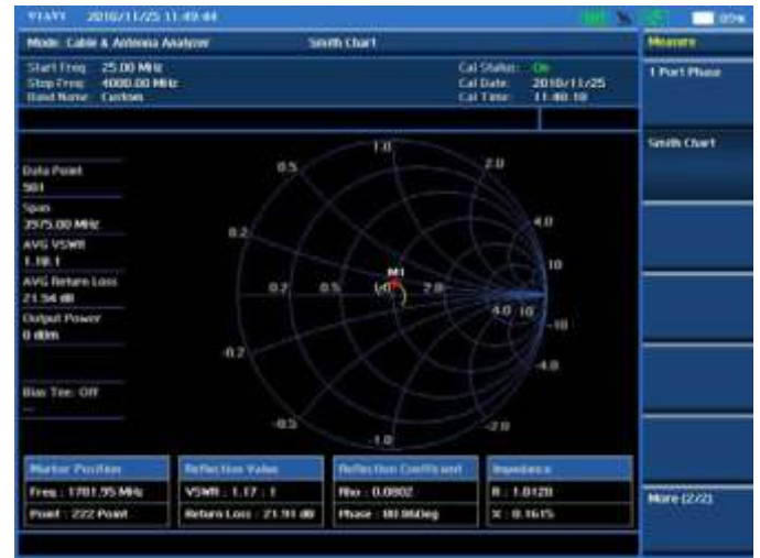
Cable and antenna test — Smith Chart
