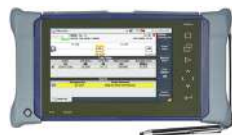
T-BERD/MTS-4000 V2 Two-slot handheld modular platform for testing fiber networks
