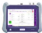
T-BERD/MTS-5800 Handheld test instrument for testing 10 G Ethernet and fiber networks
