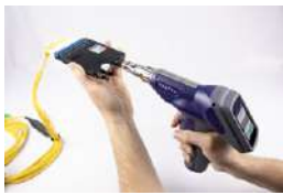
Inspect Multi-fiber Connectors
